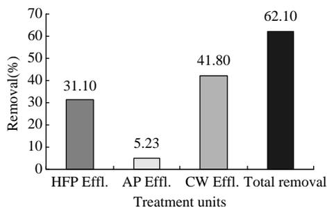
**Figure 9**  $\text{NH}_3\text{-N}$  removal in different treatment units
