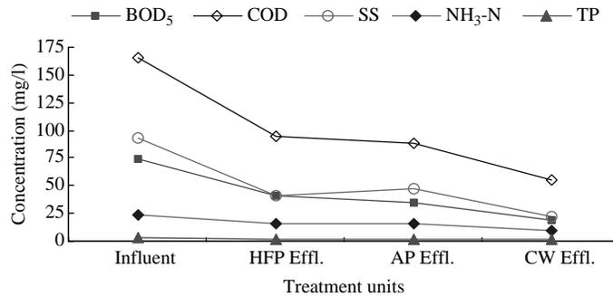
**Figure 1** Variation of main parameters along the treatment flowchart
