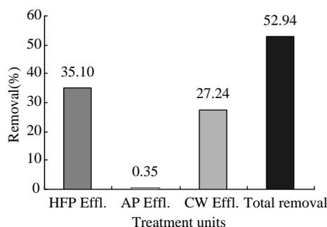
**Figure 8** TP removal in different treatment units
