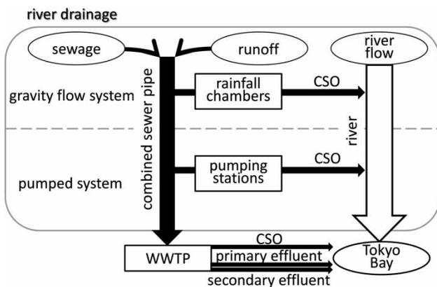
Figure 2 | Conceptual diagram of CSO discharge in combined sewer system.
