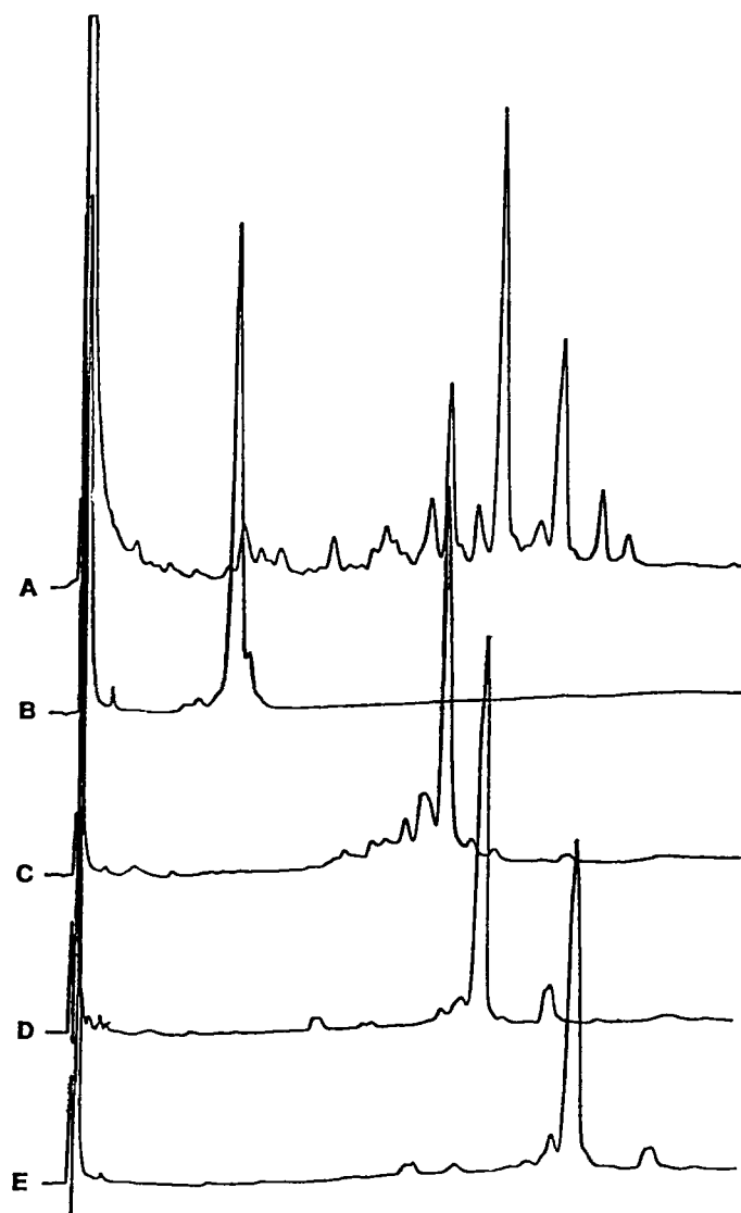
Figure 1. HPLC (Vydac C 4 , 4.6 mm \times 25 cm, 5 \mu m particle size, 3000 nm pore size) of an aqueous bark extract treated by ultrafiltration (A), saponin QS-7 (B), saponin QS-17 (C), saponin QS-18 (D), and saponin QS-21 (E). Gradient was 30 to 40% 0.1% TFA/acetonitrile/30 min, 40%/15 min at a flow rate of 1 ml/min. A total of 100 \mu g of purified saponin or 200 \mu g bark extract (dry weight) was used per injection.
