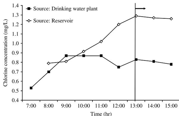
**Figure 7** | Residual chlorine concentrations at the entry points of the two distribution zones.
