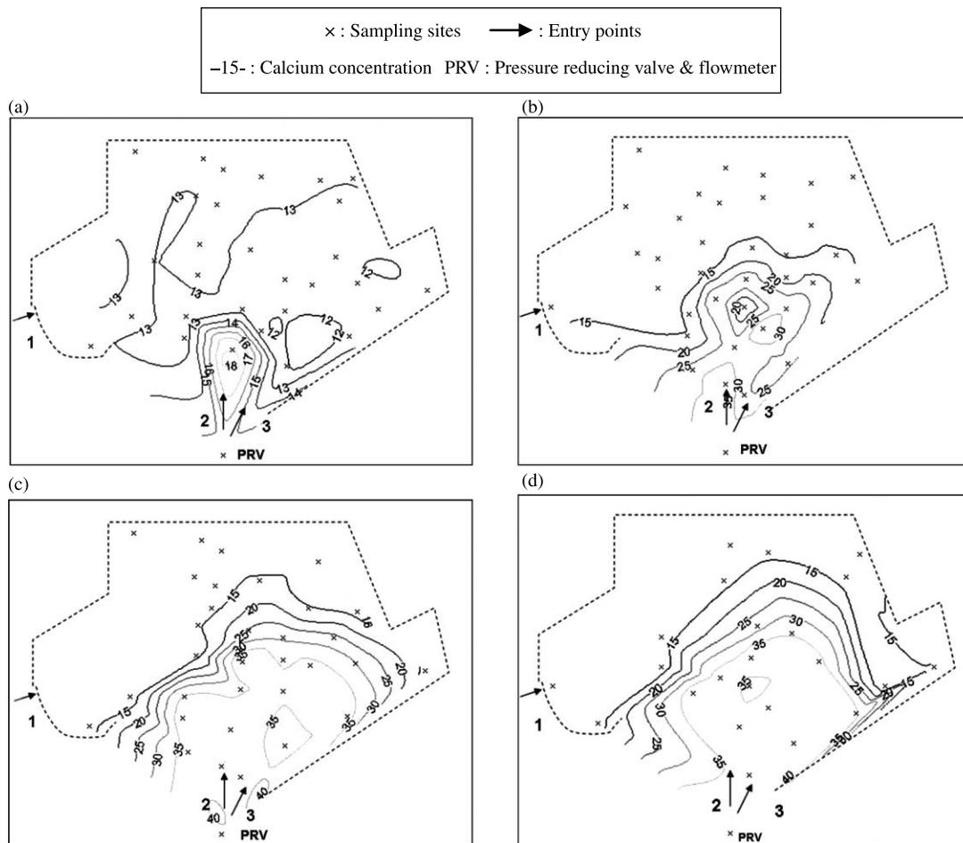
**Figure 5** | Mean measured calcium concentrations (mg/L) at sampling sites for different periods of the tracer monitoring operation: (a) 8:00–9:00; (b) 12:00–13:00; (c) 14:00–15:00; (d) 15:00–16:00.
