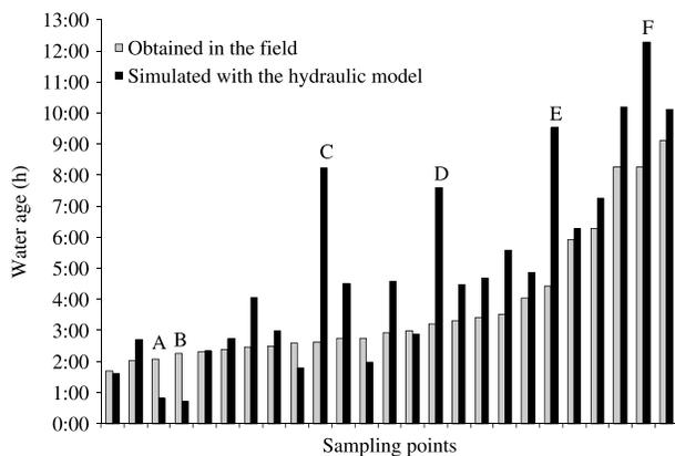
**Figure 3** | Comparison of water ages obtained in the field with those obtained from the hydraulic model. Sampling points are presented in increasing field-obtained water ages.
