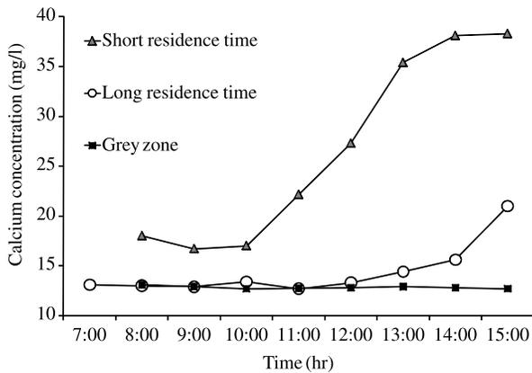
**Figure 6** | Calcium concentrations at three sampling points with different residence times.
