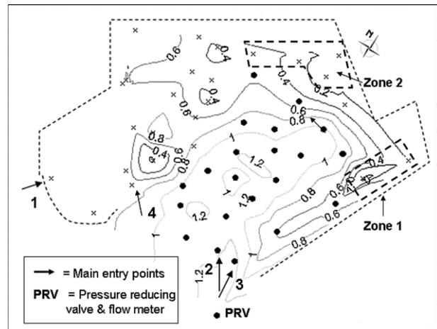
**Figure 8** | Mean residual chlorine concentrations between 14:00 and 17:00 (contour lines). Black dots represent calcium concentrations at sampling sites associated with the reservoir.
