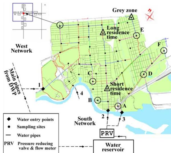
**Figure 1** | Location of inlets to the sector of interest (numbers), sampling sites (dots), sites with particular local hydraulic conditions (letters) and examples of sites with different residence times (triangles).
