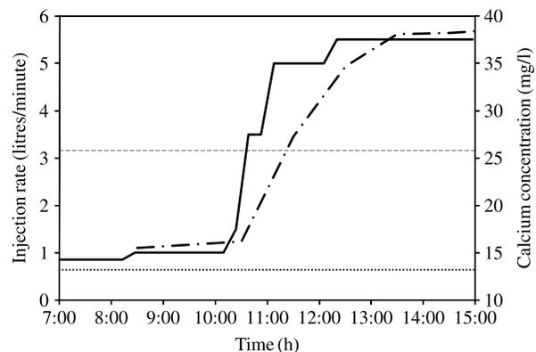
**Figure 4** | Flow rate injection of  $\text{CaCl}_2$  at the outlet of the reservoir (plain line). Broken line represents the  $\text{CaCl}_2$  concentrations at PRV chamber, dotted line represents the average DWP  $\text{CaCl}_2$  concentration and dashed line represents the mean injection rate.
