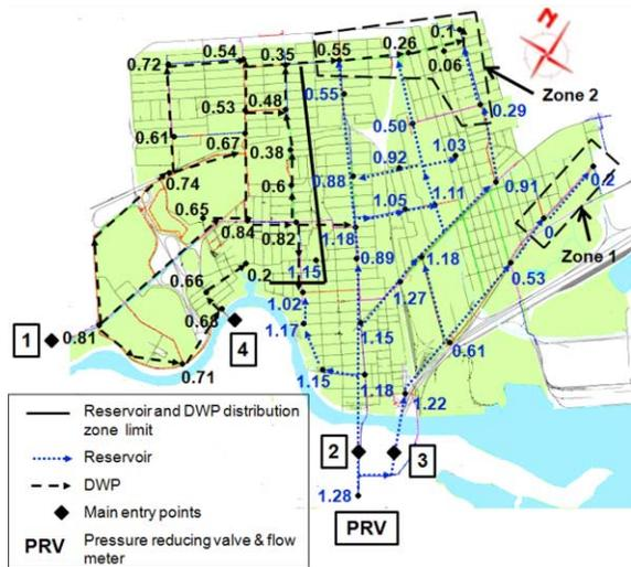
**Figure 9** | Water paths in decreasing gradients of mean residual chlorine concentrations obtained between 14:00 and 17:00.
