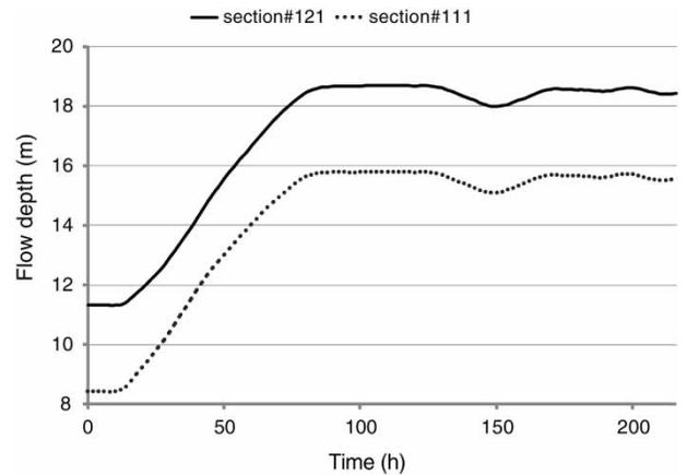
**Figure 15** | Flow depth variations during flood period at sample cross sections resulting from the PSO-Venant model.
