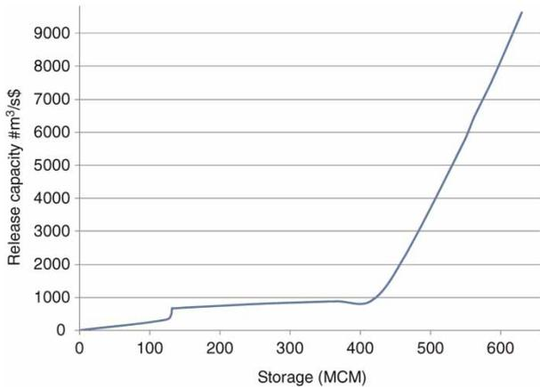
**Figure 4** | Outflow capacity curve of Bishop Dam (USACE 1998); MCM: million cubic meters.
