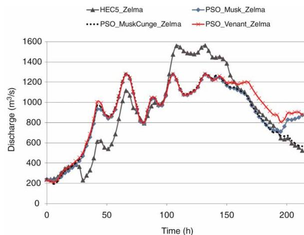
**Figure 6** | Comparison of HEC-5 and other optimization models results with respect to discharge hydrograph at Zelma control point in Bishop Dam problem.
