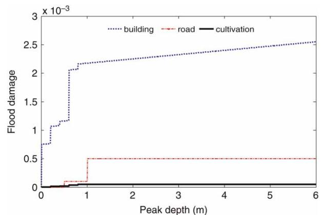
Figure 9 | Flood damage function for different types of land use data (Water Research Institute 2010).
