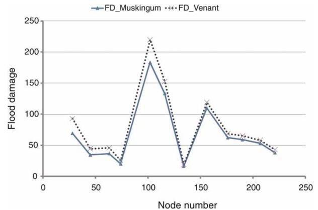
Figure 16 | Cumulated flood damage around 20 critical nodes of river.
