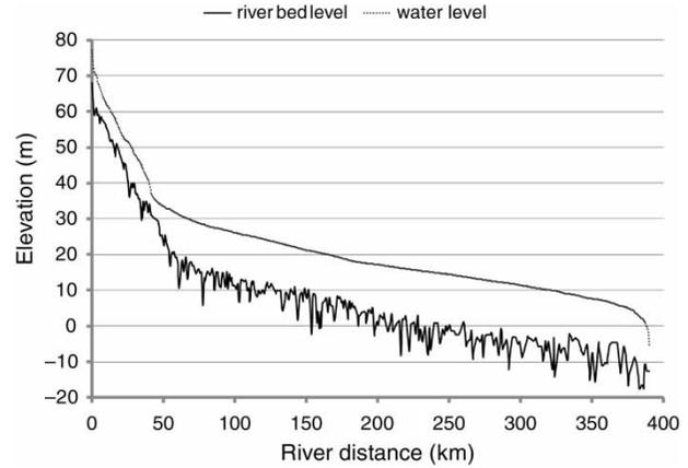
**Figure 13** | Longitudinal profile of water level in selected river reach based on best values of reservoir releases.
