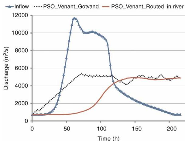
**Figure 10** | 1,000-year inflow flood hydrograph compared to optimal reservoir release hydrograph at UG dam and routed hydrograph through river reach; PSO-Venant model.
