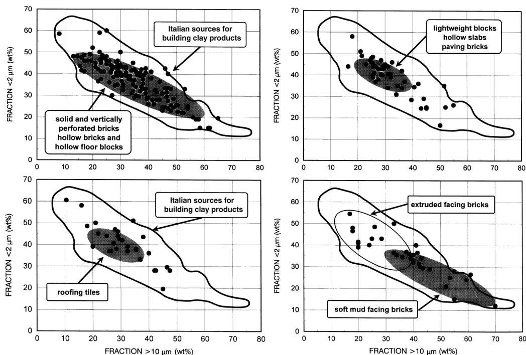
FIG. 8. Classification scheme of grain-size distribution for different types of building clay products.
