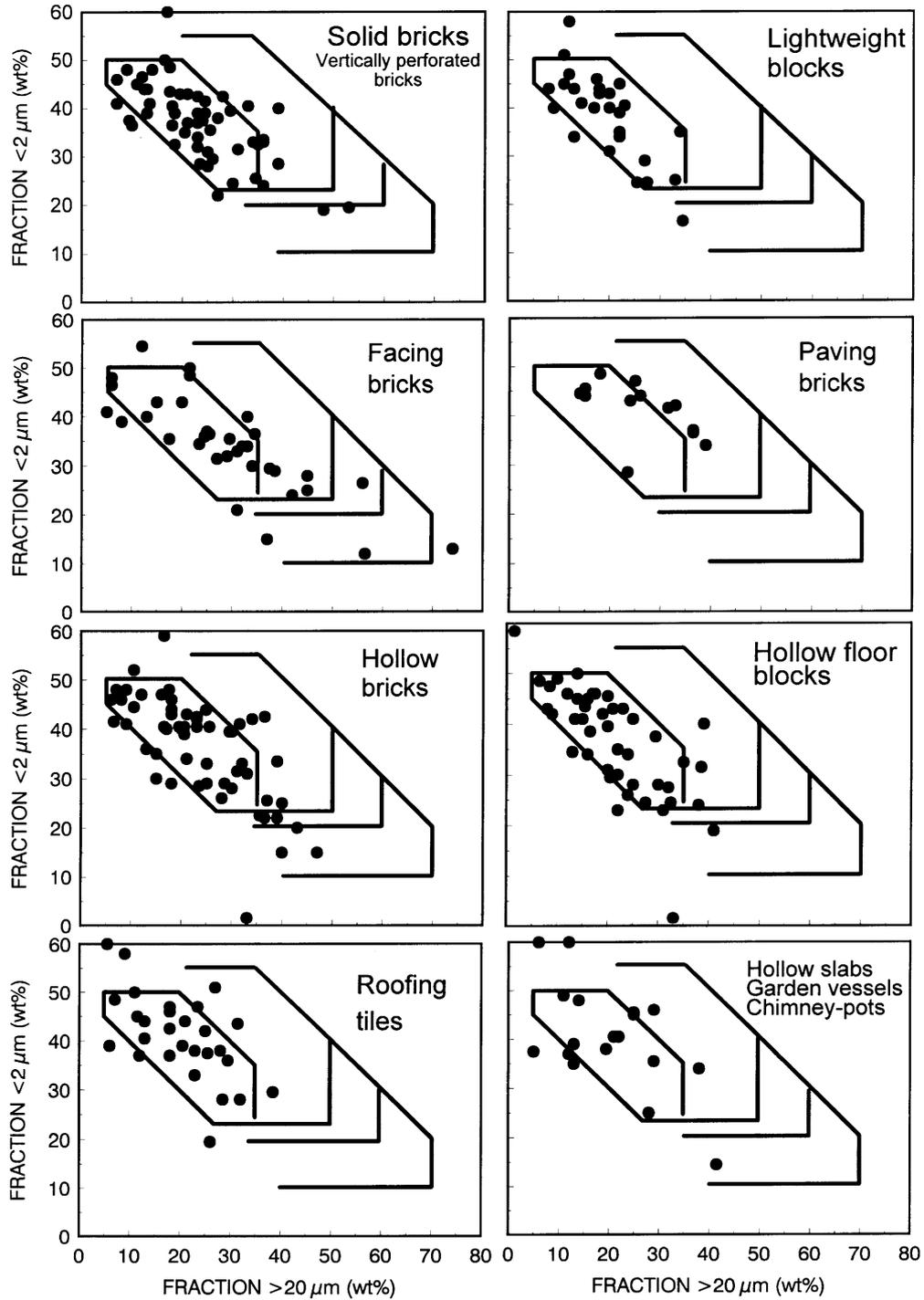
FIG. 5. Distribution in Winkler diagram of Italian bodies for different typologies of building clay products. Fields as in Fig. 2.
