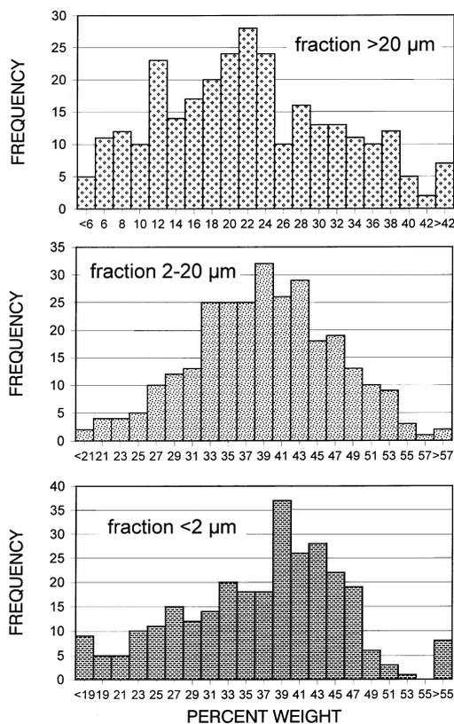
FIG. 4. Frequency distribution of three grain size fractions in the Italian bodies for building clay products.
