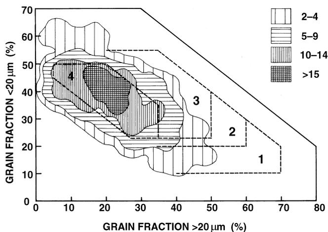
FIG. 6. Frequency distribution of Italian bodies for building clay products in a Winkler diagram. Fields 1, 2, 3 and 4 as in Fig. 2. Dashed areas represent the density of points for each percent of the surface of the diagram.
