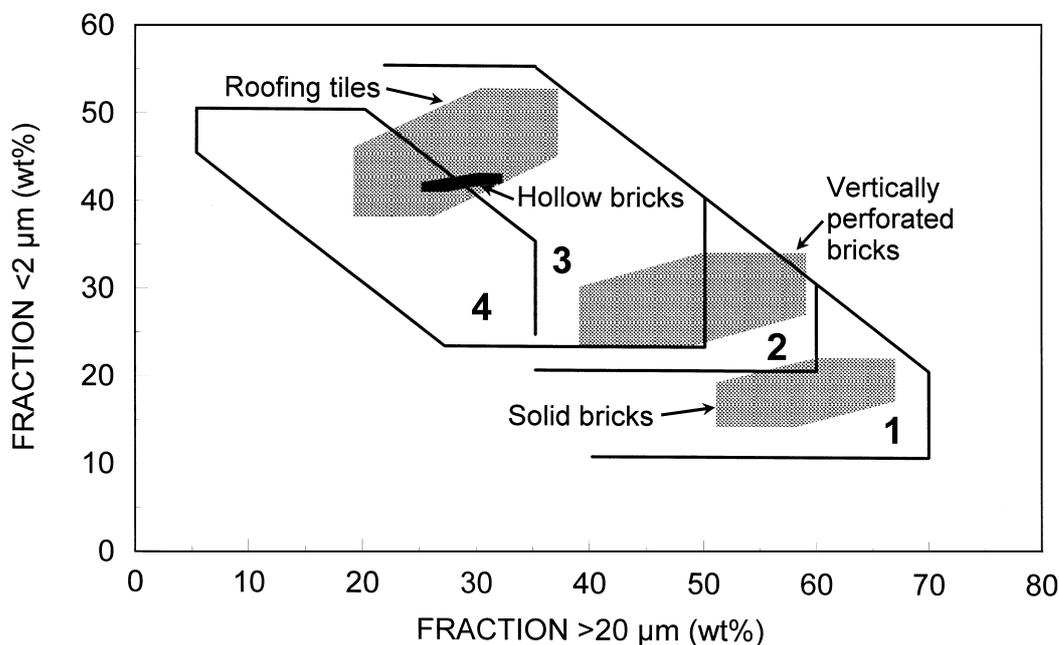
FIG. 7. Typical grain-size distribution for different typologies of German building clay products (Schmidt-Reinholz, 1993) in comparison with Winkler fields (1, 2, 3 and 4 as in Fig. 2).
