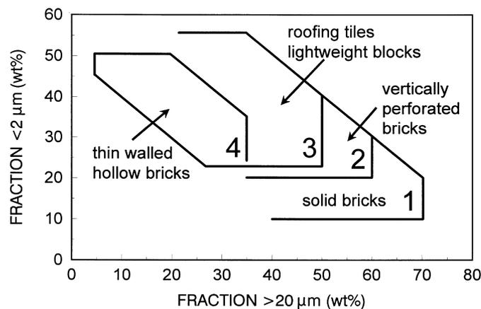
FIG. 2. Winkler diagram (Winkler, 1954) for the technological classification of bodies for structural clay products.
