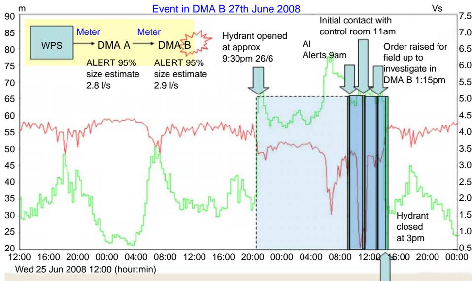
Figure 5 | Event 2—Hydrant flushing event detection in DMA B (25th to 27th June 2008).
