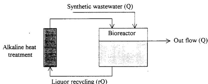
**Figure 1** Configuration of the laboratory pilot plant. The bioreactor was operating as a chemostat with a hydraulic dilution rate of  $0.02 \text{ h}^{-1}$ . The alkaline heat treatment reactor was coupled to the bioreactor.
