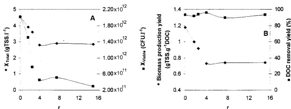
**Figure 4** Steady state results of the laboratory pilot plant operating at various liquor recycling rates ( $r$  between 0 and 15). The bioreactor was fed with a synthetic wastewater ( $3.9 \text{ gDOC.l}^{-1}$  of acetate, flow rate  $Q = 0.061 \text{ l.h}^{-1}$ ) and the alkaline heat treatment reactor was maintained at  $60^\circ\text{C}$  and pH 10 (NaOH addition) with a liquor residence time of 20 min
