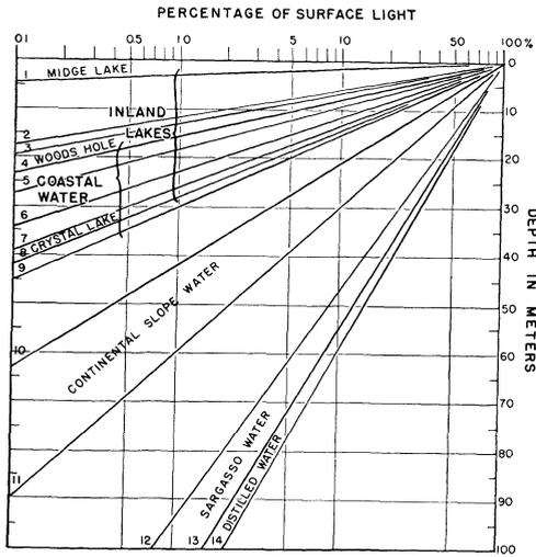
FIGURE 3. Comparison of the rates of penetration of the yellow-green component of daylight into natural waters. Curves show the relation between depth and illumination expressed as a percentage of the light at the surface. (Logarithmic scale.)
