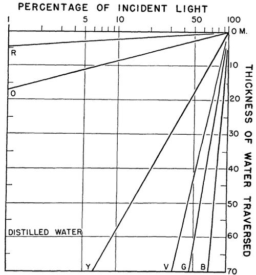
FIGURE 1. Transmission of light by distilled water at six wavelengths within the visible spectrum. Curves show the percentage of incident light (logarithmic scale) which would remain after passing through the indicated thickness of water.
