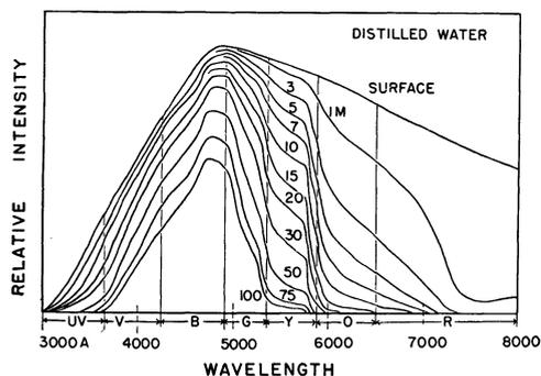
FIGURE 2. The spectral distribution of solar energy at the earth's surface is given by the uppermost curve. When sunlight is passed through successive meters of pure (distilled) water, the reduction of intensity and the change in spectral distribution which result are indicated by the curves beneath. (Courtesy of Dr. E. A. Birge.)
