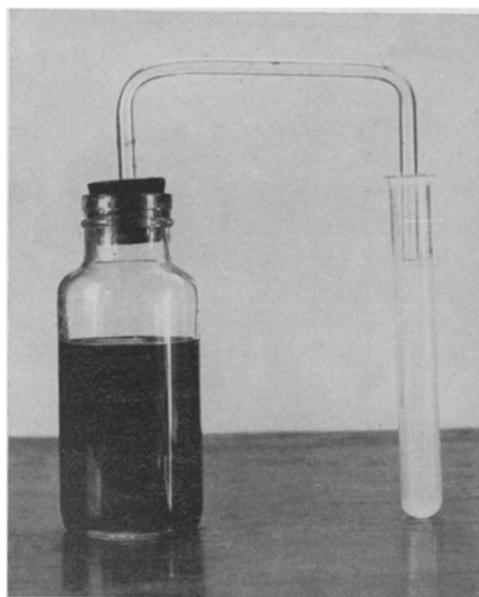
Figure 2. Gas forced through the glass tube will bubble through the limewater in the test tube and cause a milky deposit.
