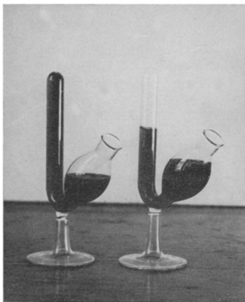
Figure 1. Left: at the beginning of the experiment; right: after an interval depending on room temperature the gas resulting from the fermentation process has collected in the closed arm of the fermentation tube.
