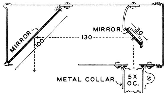
A simple microprojector made from two front-silvered mirrors and a metal mailing tube can be used for drawing or measuring at table level.
