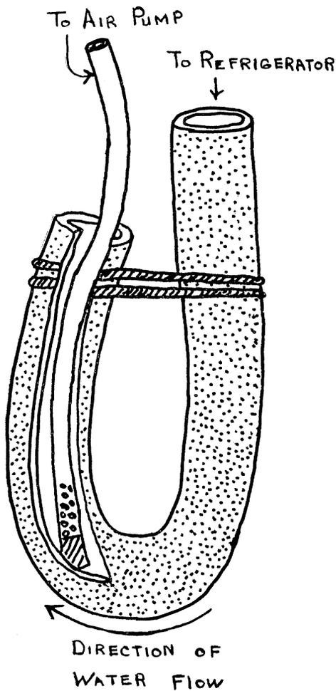
Fig. 2. Cutaway view of bubble pump used to circulate water.
