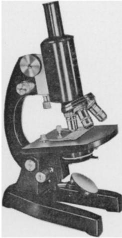
59-1160 **Biological Microscope WK3.** Wolfe. Monocular. Equipped with 10X Huyghenian pointer eyepiece, 10X (N.A. 0.30) and 45X (N.A. 0.65) parfocal achromatic objectives, spring-loaded 100X (N.A. 1.30) oil immersion achromatic objective, oversize stage and stage clips, N.A. 1.40 Abbe condenser with rack and pinion, iris diaphragm, filter holder, and plano-concave mirror. With plastic dust cover.
