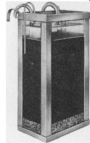
Rugged stainless steel and plate glass unit hangs on the side of an aquarium or remains free-standing on nearby flat surfaces. Water is siphoned into the top of the filter, harmful waste material is removed, and purified water is returned automatically to the aquarium by very efficient air lift.
