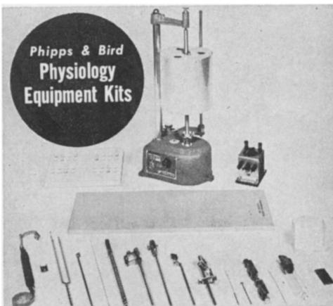
A kit of physiology equipment has been assembled as a teaching aid for the rapidly expanding field of biological science. This kit, housed in a durable metal valise type case, allows the student to perform a variety of the basic physiology experiments. There are three models: the PK#1 for smoke writing; the PK#2 is identical to the PK#1 except a Smoking Stand and Burner is included; and the PK#3 for ink writing.
