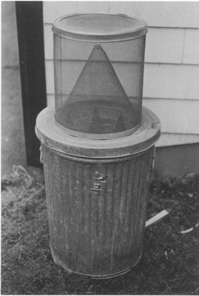
Fig. 1. Garbage can fitted with a screen trap for collecting flies.
