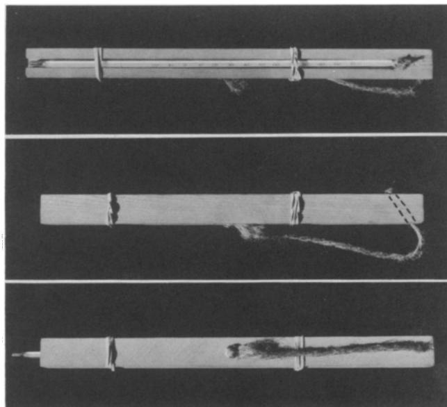
Front, side, and rear views of the thermometer guard. Side view shows direction of bore for loop string.
