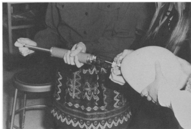
Fig. 2. Transferring sample to indicator tube by means of gas-detector pump.
