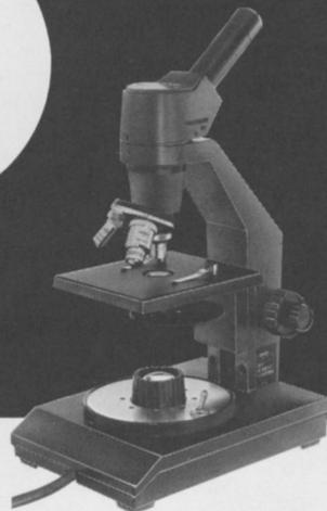
Patented safety features assure years of service for these scientifically engineered SWIFT microscopes. Modular concept provides for every teaching requirement. Focusing stage is constantly horizontal. Built-in slip clutch prevents gear damage. Other features include: widefield W 10x eyepiece, built-in illuminator, brightfield at all magnifications, phase contrast at 100x-400x, darkfield at 40x.
