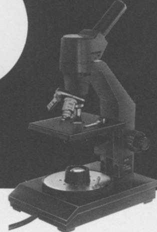
Patented safety features assure years of service for these scientifically engineered SWIFT microscopes. Modular concept provides for every teaching requirement. Focusing stage is constantly horizontal. Built-in slip clutch prevents gear damage. Other features include: widefield W 10x eyepiece, built-in illuminator, brightfield at all magnifications, phase contrast at 100x-400x, darkfield at 40x.
