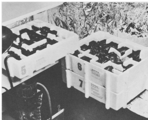
**Fig. 5.** In stages 5 and 6 the algae, in tanks, convert the nitrates. In stage 7 the algae are prevented from entering the specimen tank. Lights burn continuously above the tanks, to promote algal reproduction.
