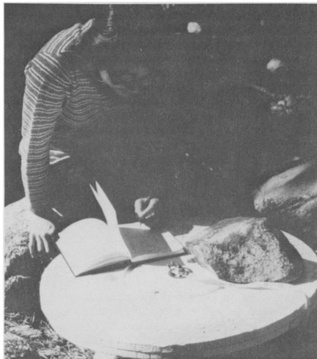
**Fig. 2.** A giant protractor made of half of a large wire spool was used to determine the distance and angle of each tree or group of saplings from a fixed corner of the plot.
