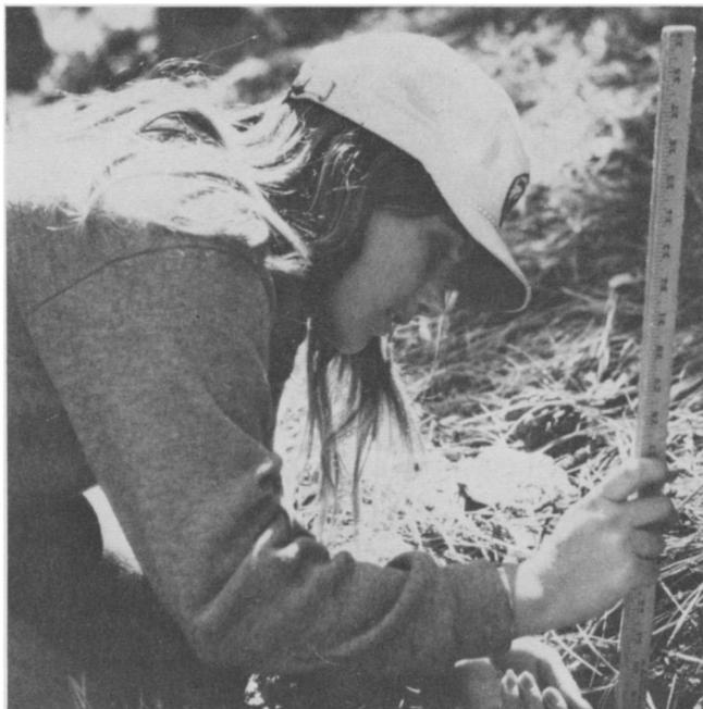
**Fig. 1.** Litter and duff accumulation was measured to determine total flash-fuel levels before burning.
