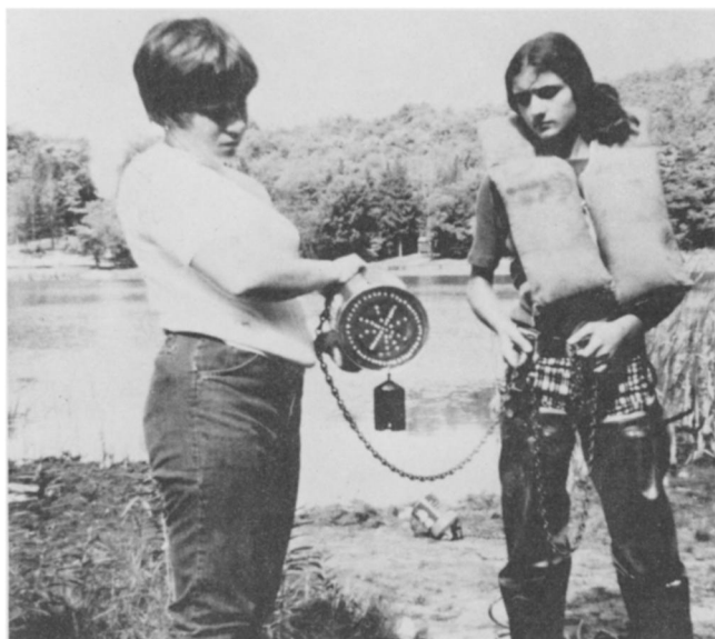
Fig. 3. In the foreground, students examine a bottom sampler (dredge). On the ground near the water note the plankton net.
