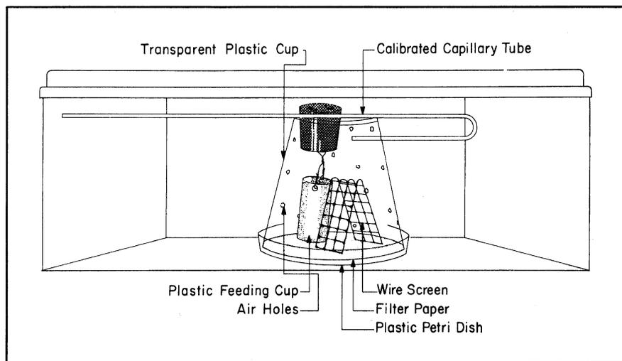
FIGURE 1. A front view of the chamber and cage suitable for use in insect studies.
