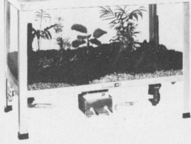
Chamber shown with optional pump for circulating gases.
