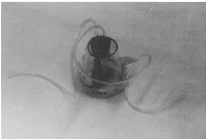
FIGURE 2. Insertion of rubber-stopper apparatus into flower pot assembly.
