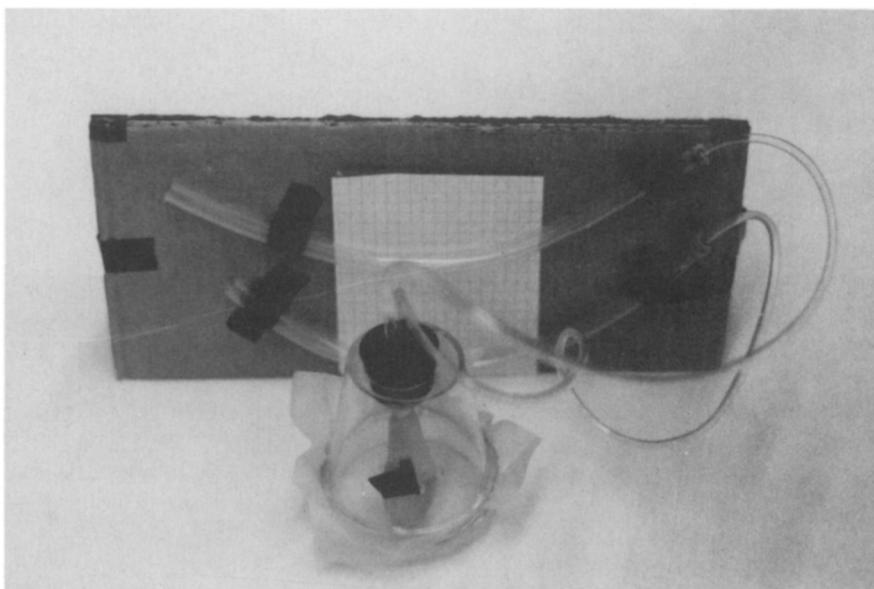
FIGURE 3. Model completely assembled. It can be used for manometric measurements. The curved tube contains colored water to illustrate pressure changes as the diaphragm is moved.
