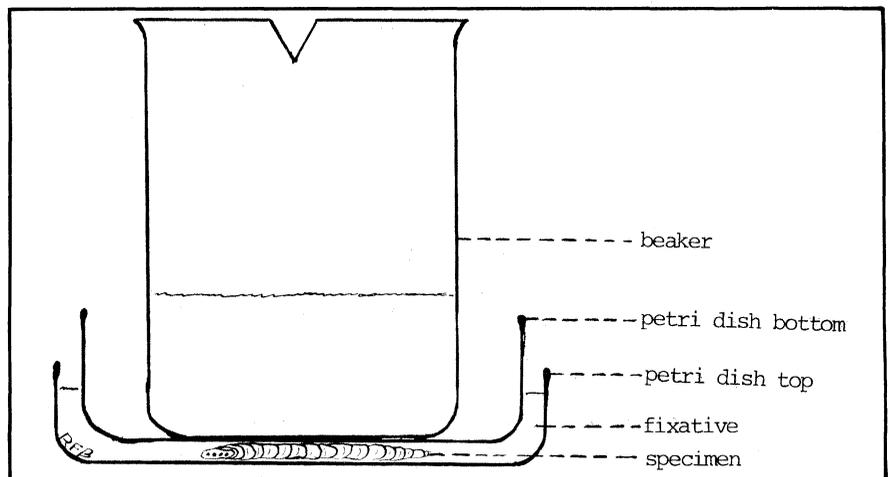
FIGURE 1. Worm-flattening device described in this article.
