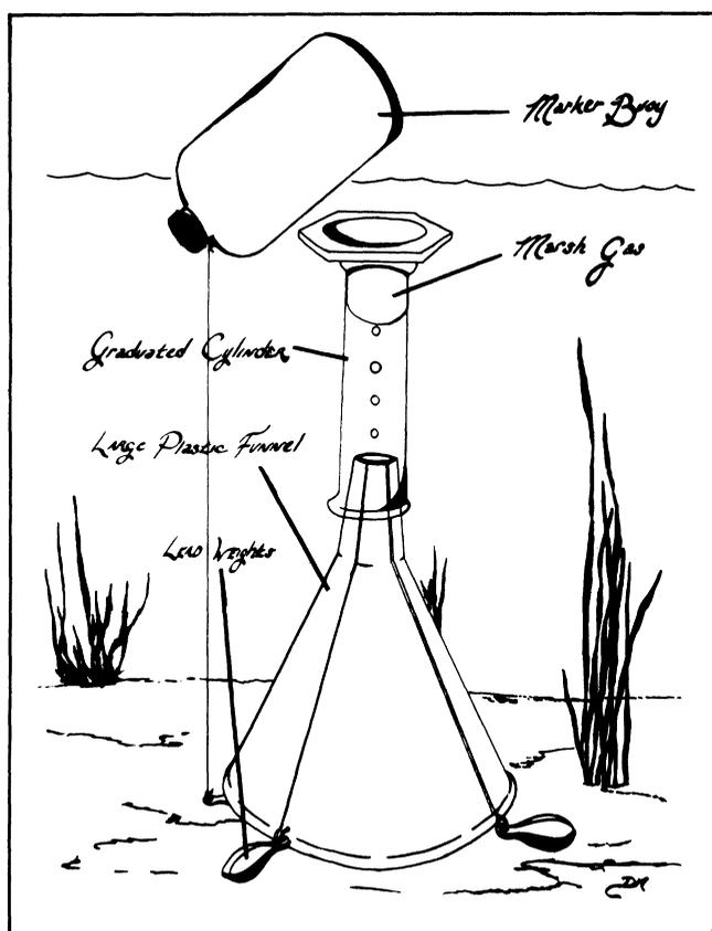
FIGURE 2. Apparatus demonstrating marsh gas production from fresh or salt water sediments. (Drawings by Dana Carpenter.)
