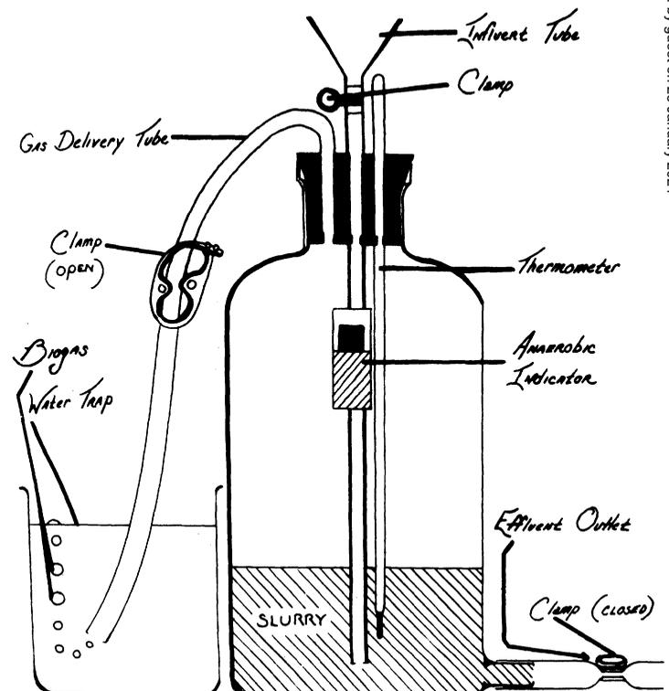
FIGURE 7. A methane digester assembled from an aspirator bottle facilitates sampling of the slurry.
