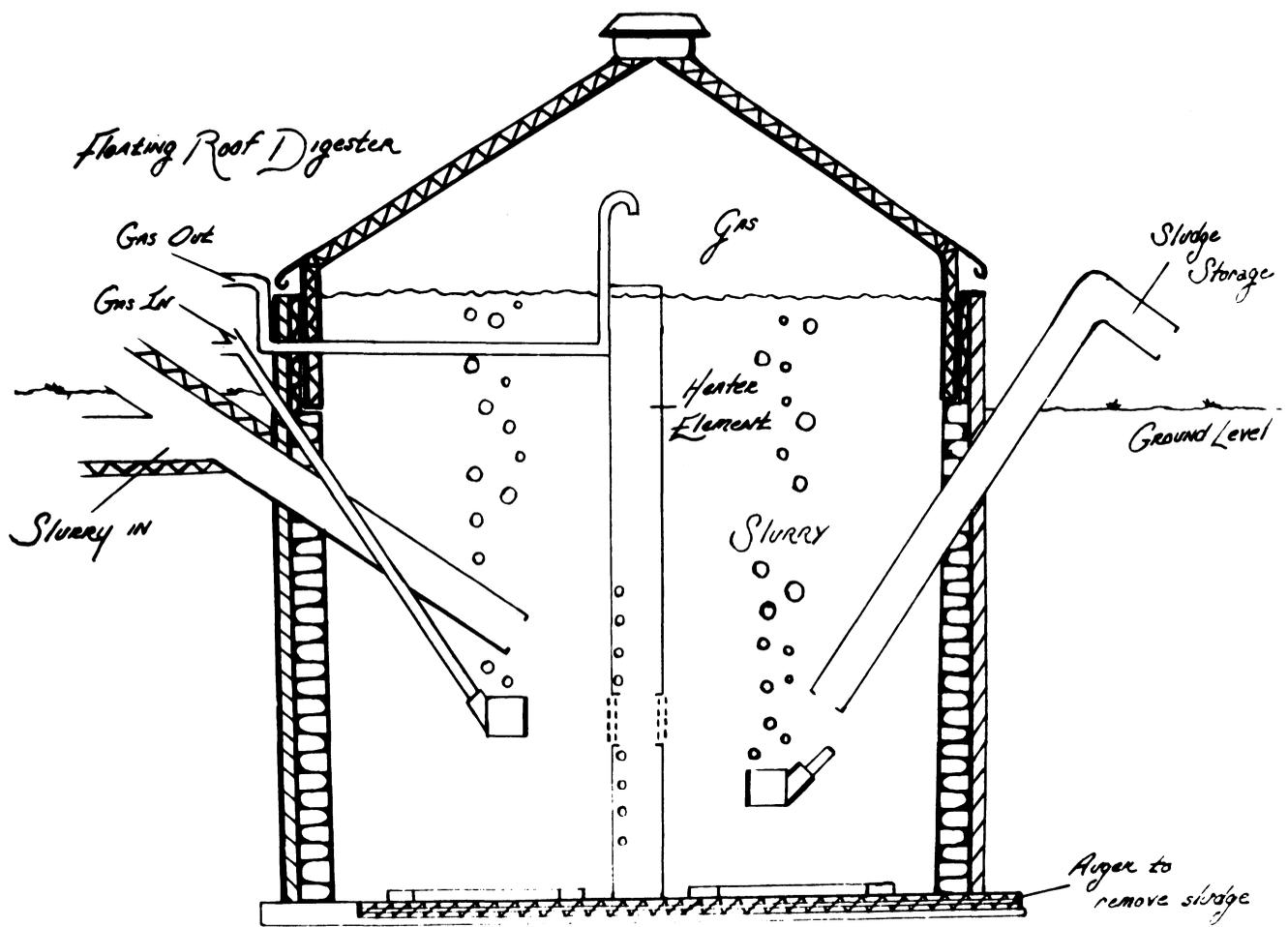
FIGURE 4. A floating roof methane digester. Adapted with permission from P.S.U. College of Agriculture Extension Service, Special Circular 260.
