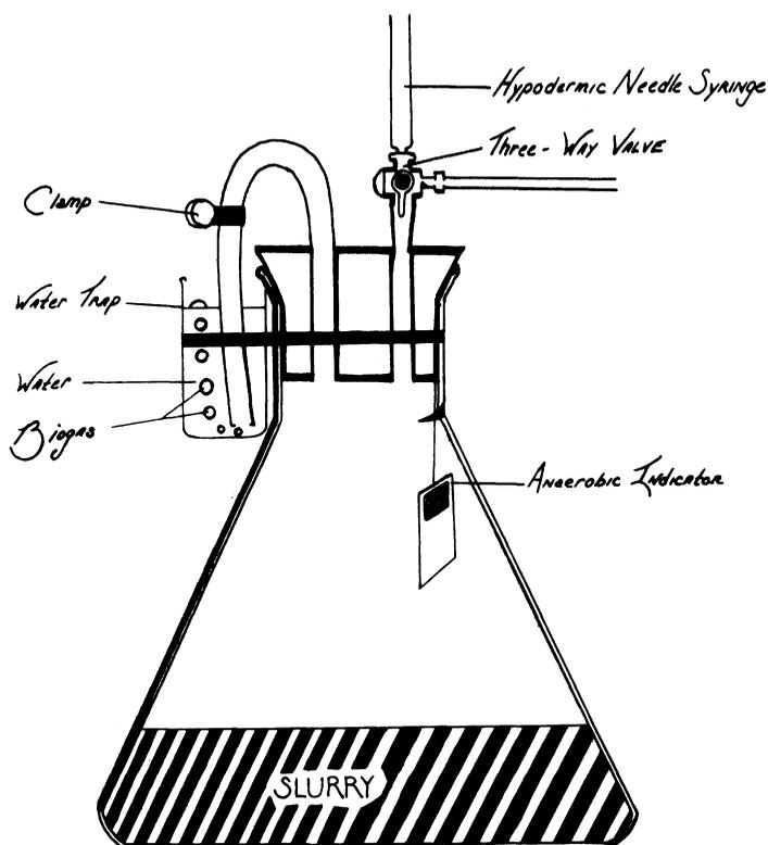
FIGURE 6. Simple methane digester assembled using a 1 liter Erlenmeyer flask.
