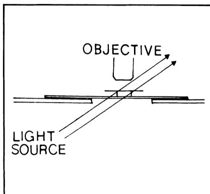
FIGURE 4. Dark-field illumination without a condenser. Light source is positioned to the side of the specimen so that no light enters the objective lens directly (arrows). Only light reflected or refracted by the specimen will enter the objective.
