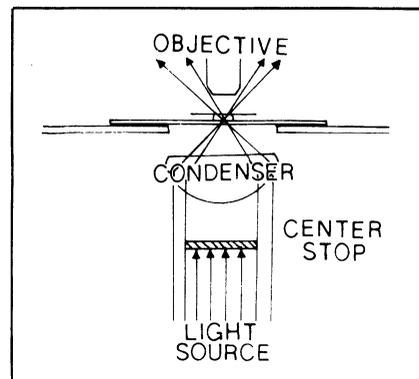
FIGURE 5. Dark-field illumination with a condenser lens. An opaque filter, the center stop, is placed in the light path below the condenser so that no light will pass directly into the objective (arrows). Only light reflected or refracted by the specimen will enter the objective lens.
