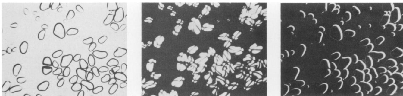
FIGURES 6-8. Starch grains seen with various types of light microscopy. All photomicrographs were made of the same preparation using a standard student microscope and techniques outlined in this paper. Fig. 6. Image with standard bright-field illumination. Fig. 7. Image using polarization microscopy. Fig. 8. Image using dark-field microscopy.
