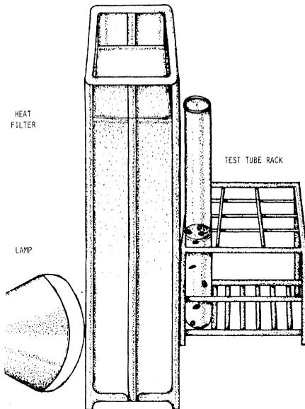
FIGURE 2. Arrangements of the lamp, heat filter, and test tube rack for a photosynthesis assay. The bottom of the test tube should be situated adjacent to the center of the lamp.
