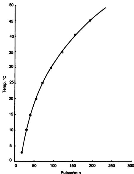
Figure 1. Typical transmitter calibration curve.
