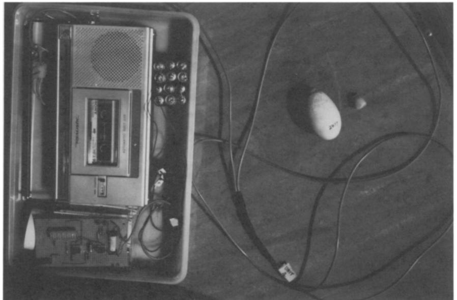
Figure 3. A complete system for gathering incubation data. The radio, timer and battery pack are placed in a moisture proof plastic cake pan.
