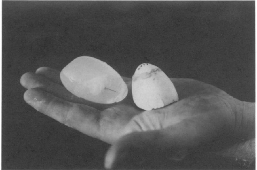
Figure 2. Transmitter suspended in agar gel. Note the egg shell with the epoxied end.
