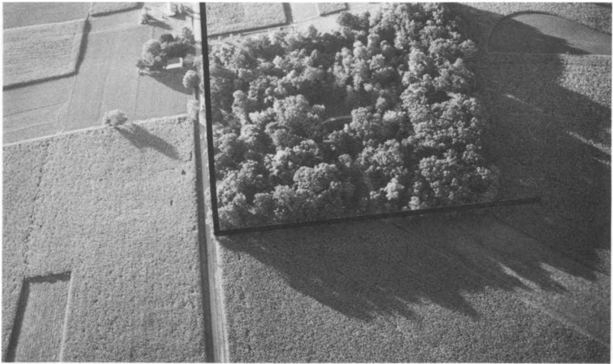
Figure 4. Aerial photograph of a small wooded plot in Lancaster County, Pennsylvania, with two axes superimposed on the photograph to illustrate how random samples could be located in this wooded area.
