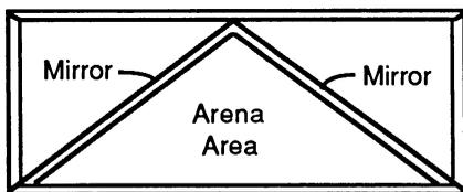
Figure 2. Top view of a modified aquarium used in an arena for video recording *Peromyscus* behavior. The mirrors may be placed at any suitable angle which permits viewing the subject from all sides simultaneously.
