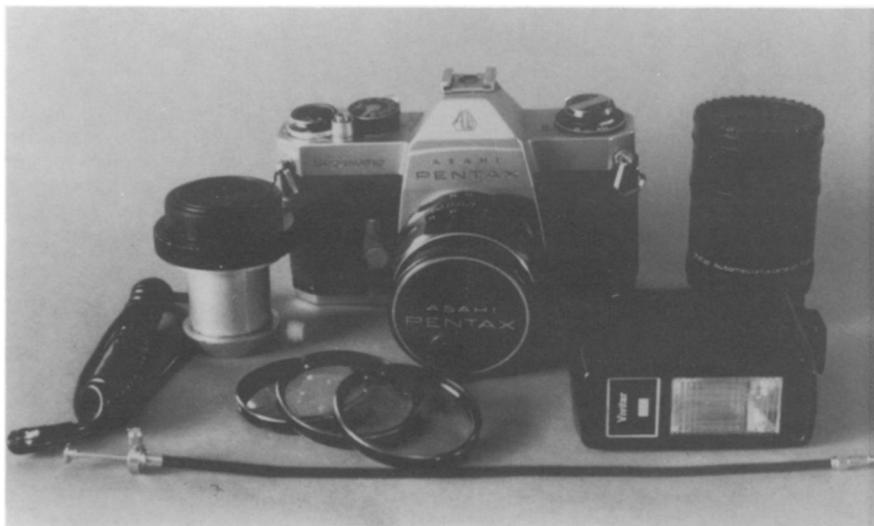
Basic equipment for classroom photography (from left to right) back row: microscope adapter, camera, extension tubes; front row: flash cord, close-up lenses, flash, and cable release.
