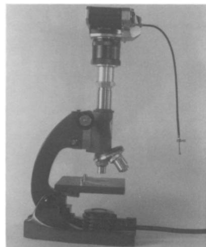
Camera adapted to a microscope, ready for photography. Note: by adding a 36mm extension tube between the camera body and the microscope adapter, full frame pictures are possible.
