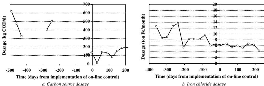
**Figure 5** Effect of on-line control on chemicals dosing
