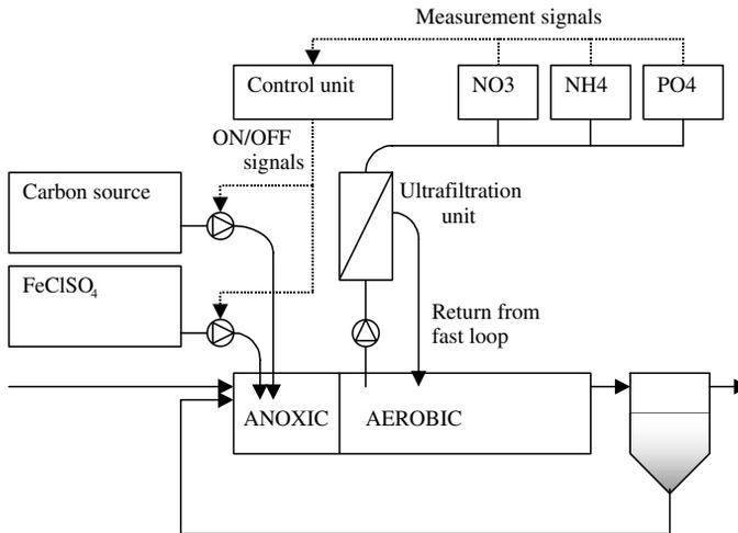
**Figure 2** Implantation of the control strategy at the plant
