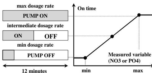
**Figure 3** Principle of the proportional controllers
