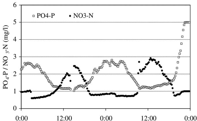
**Figure 1** Example of daily variability: nitrate and phosphate concentration in the aeration tank during two consecutive days
