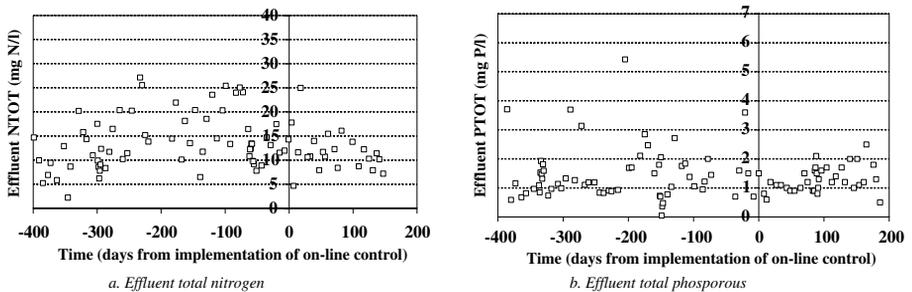
**Figure 4** Effect of on-line control on effluent results
