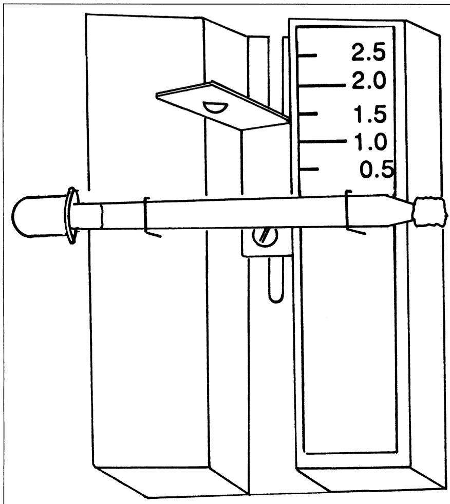
Figure 1. Completed van Leeuwenhoek microscope (not to scale).
