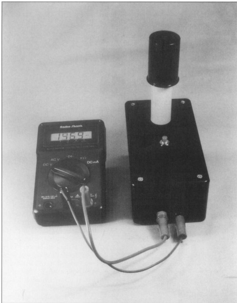
Figure 1. Photometer connected to voltmeter.
