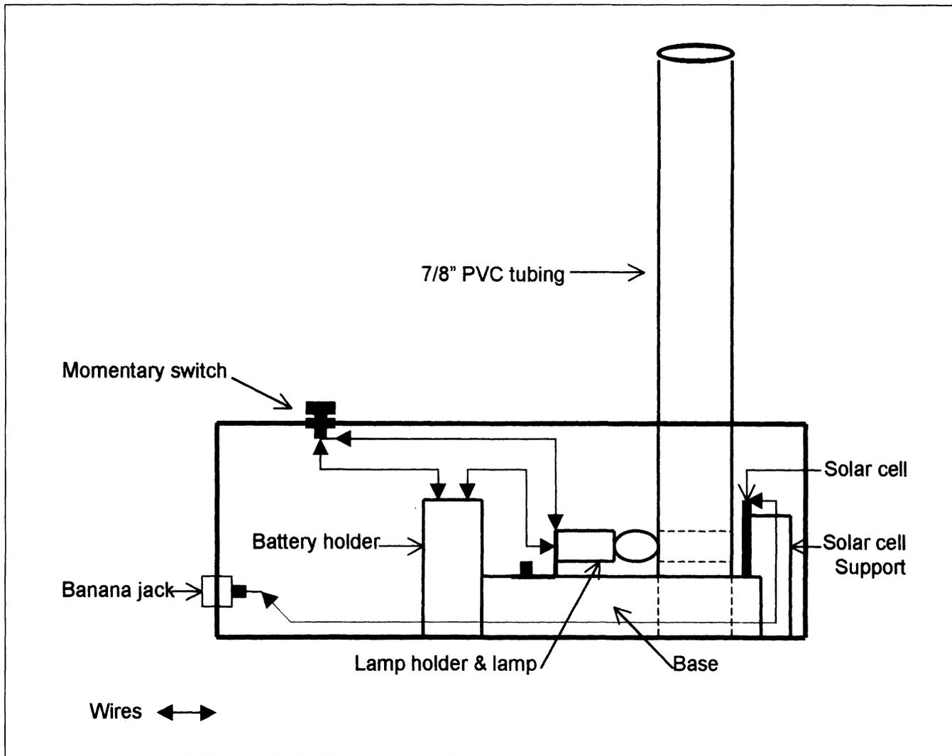
Figure 3. Photometer in phantom side view.
