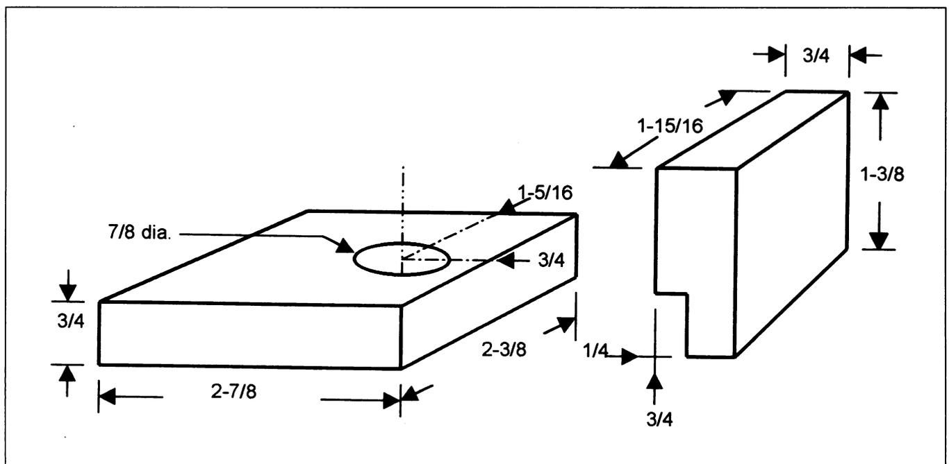
Figure 2. Base (left) and solar cell support (right). Both pieces are cut from 1-inch stock boards. All measurements are in inches.
