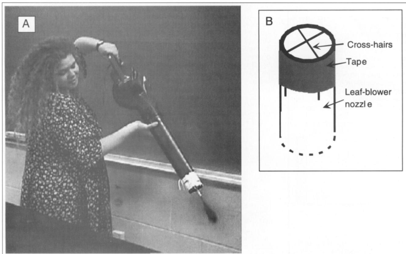
Figure 1A. A student demonstrates the leaf blower experimental system. 1B. Diagram of leaf blower exit nozzle showing cross hairs attached with tape.
