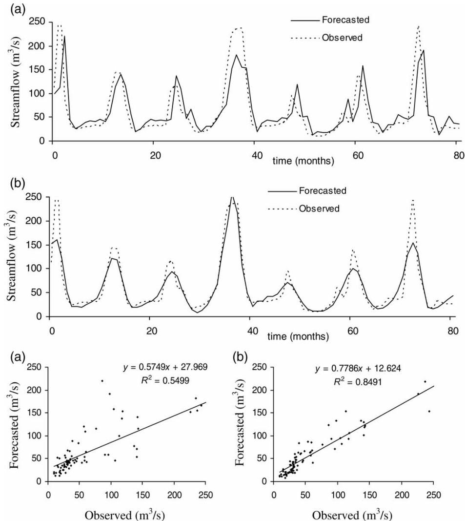
**Figure 3** | Observed and forecasted streamflow using (a) neuro-fuzzy and (b) wavelet-neuro-fuzzy model at station 1413 for test period.
