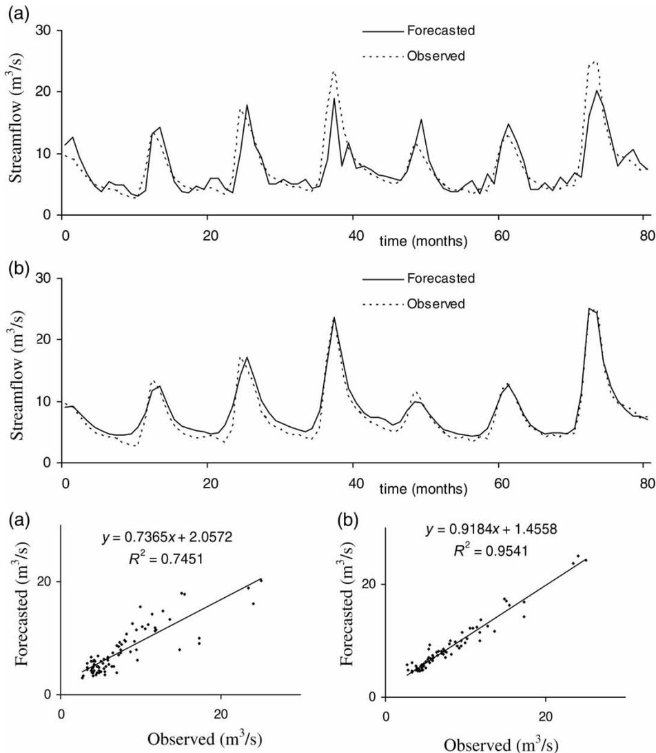
**Figure 4** | Observed and forecasted streamflow using (a) neuro-fuzzy and (b) wavelet-neuro-fuzzy model at station 2015 for test period.
