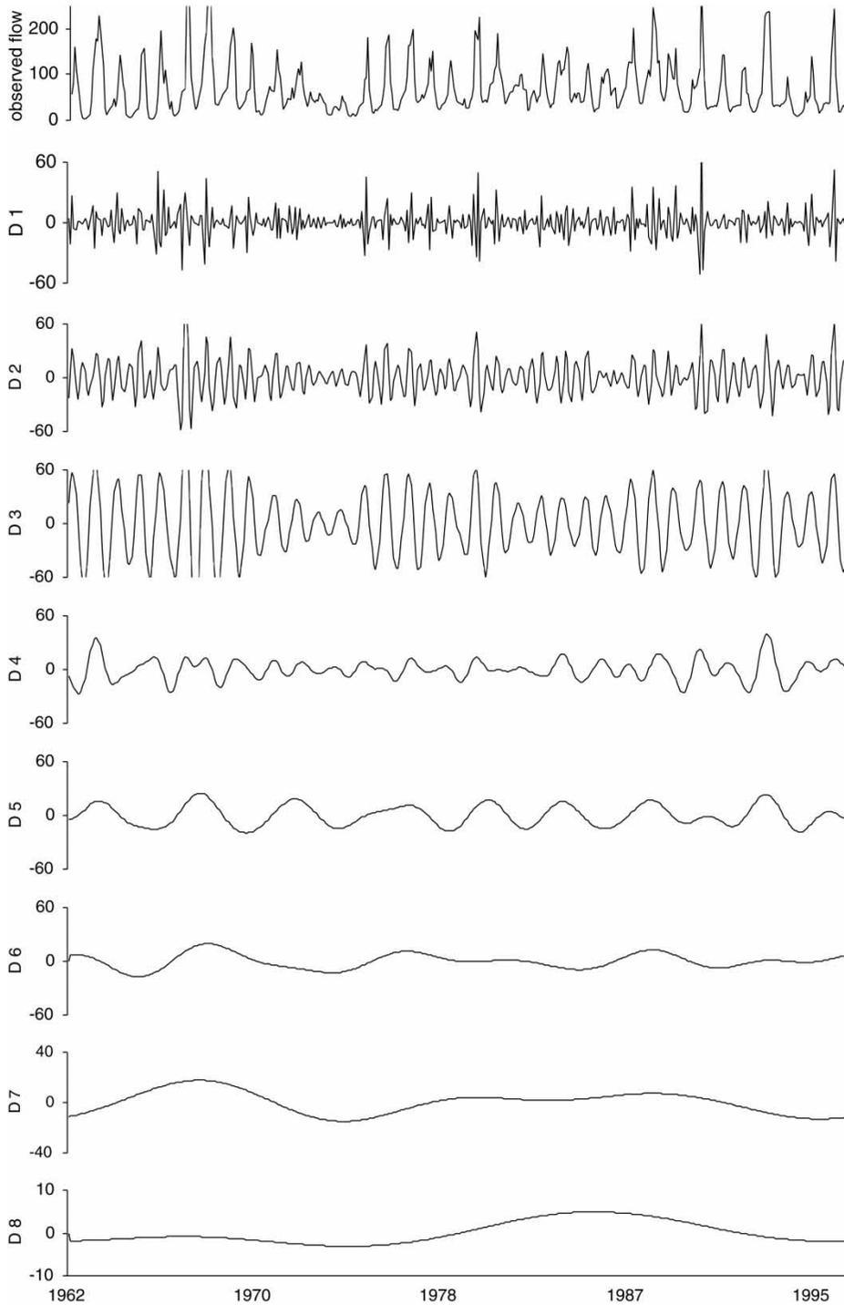
**Figure 2** | Decomposed wavelet sub-time series at station 1413.
