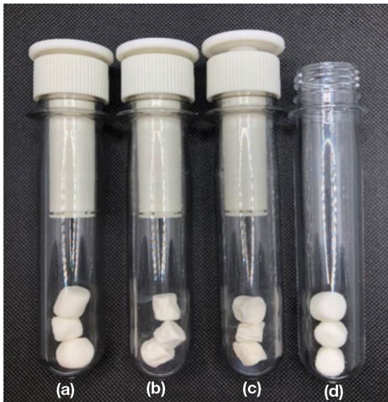
Fig. 1. (a)–(c) Marshmallows in unpumped (a), moderately pumped (b), and highly pumped (c) tubes. (d) The marshmallows return to their original shape when the pump is removed.
