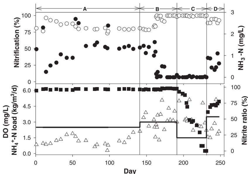
**Figure 1** Profiles of free ammonia ( $\text{NH}_3\text{-N}$ , ●), dissolved oxygen ( $\Delta$ ), Nitrification efficiency ( $\circ$ ),  $\text{NH}_4^+\text{-N}$  load (—), and Nitrite ratio (■) as function of time in the biofilm airlift reactor
