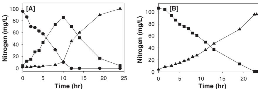
**Figure 2** Batch nitrification kinetic analysis of nitrite accumulating biofilm from the biofilm airlift reactor ([A]: ammonia oxidation, [B]: nitrite oxidation, (●:  $\text{NH}_4^+\text{-N}$ ; ■:  $\text{NO}_2^-\text{-N}$ ; ▲:  $\text{NO}_3^-\text{-N}$ ))
