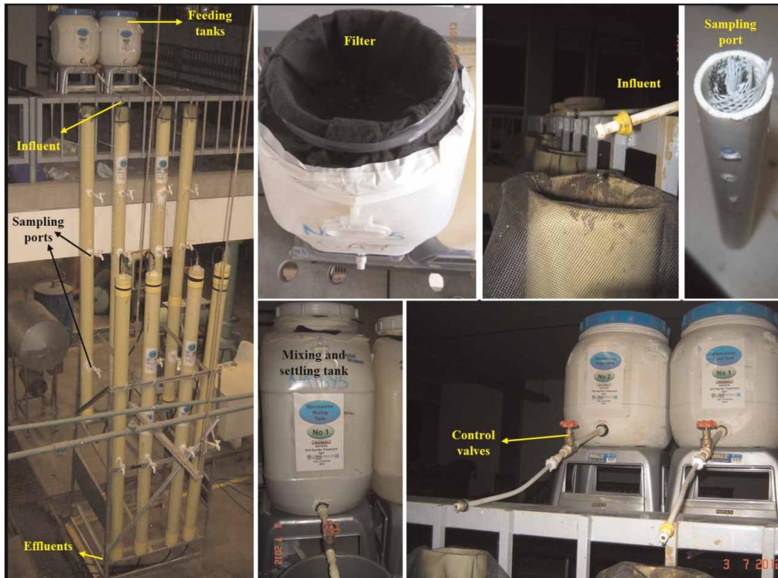
Figure 1 | Pilot-scale SAT experimental set-up used.
