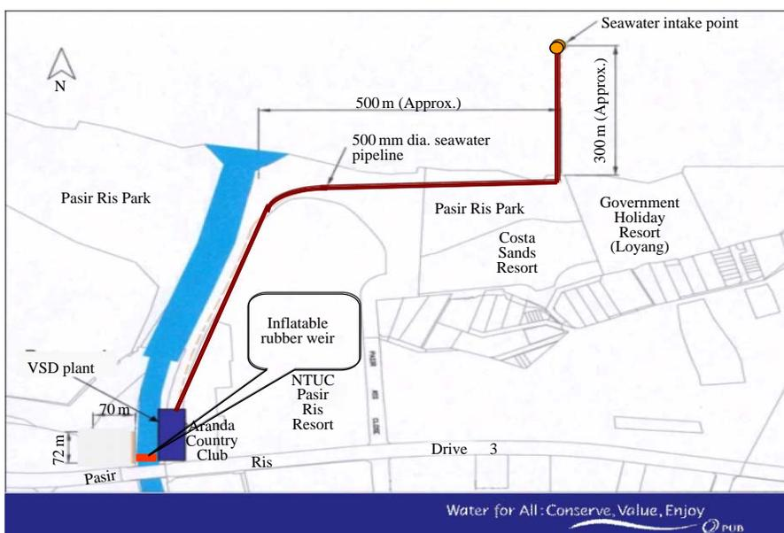
Figure 1 | Site plan of variable salinity desalination plant at Tampines River.
