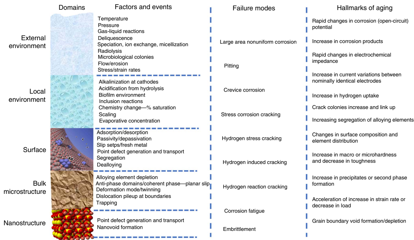
FIGURE 7. Domains of metallic alloy corrosion with processes at different size scales and hallmarks of aging leading to observable failure modes.
