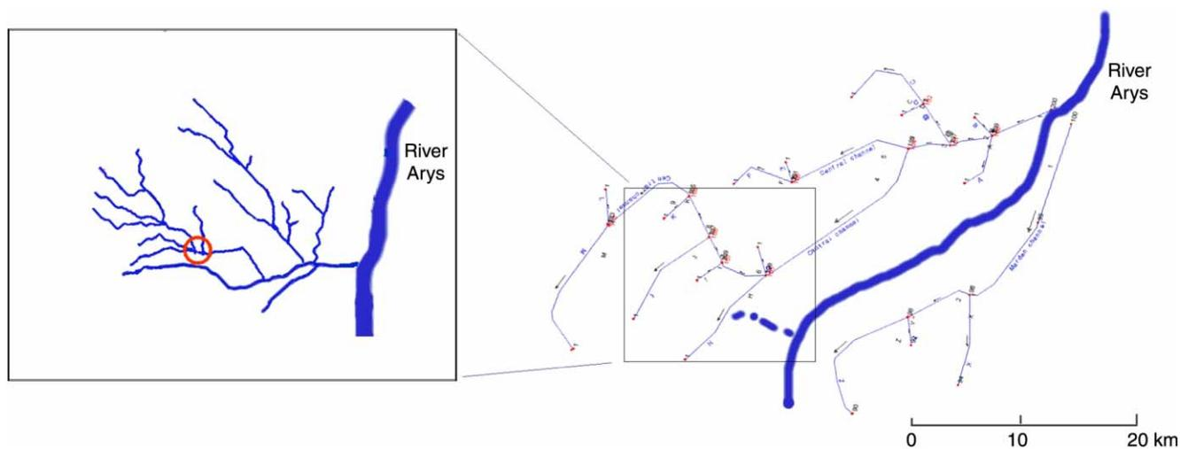
**Figure 8** | HEC RAS model of the 12th century system (left) in relation to the modern day canal network (right). Broken line indicates original offtake from the river into the canal network. Circle shows location of the “Altyn Knot”.
