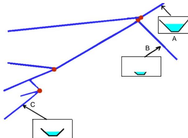
**Figure 9** | Simulation of 12th century water distribution system with no control gates. A=main canal input, B=small canal over flowing, C=large canal receiving too little water.
