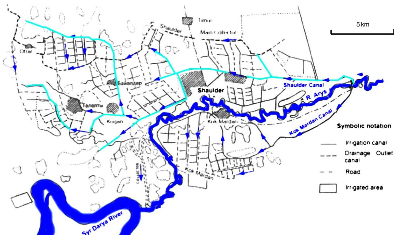
Figure 11 | Modern irrigation system layout.
