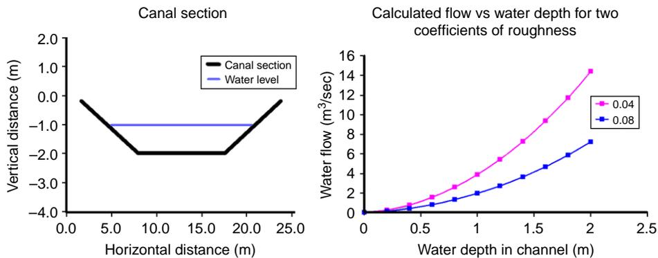
**Figure 6** | Use of canal cross section data to estimate water carrying capacity using Manning's equation.
