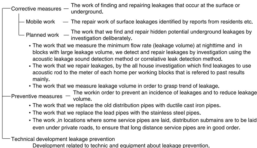
Figure 7 | System of leakage prevention measures.
