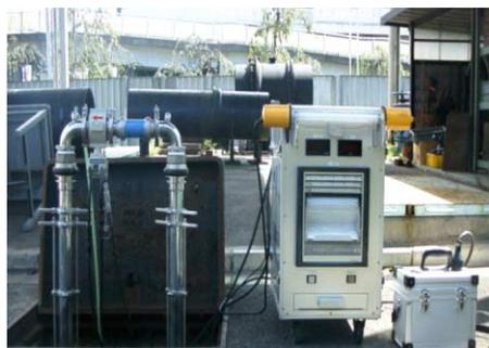
**Figure 8** | Portable minimum flow meter.
