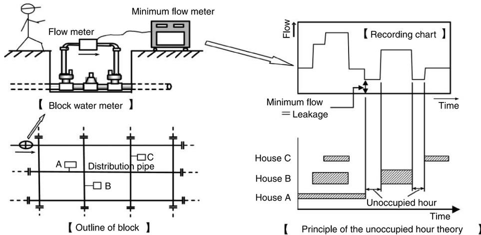
Figure 2 | Theory of minimum night flow measurement method.
