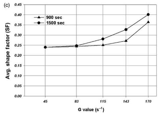
**Figure 4** | Feret Diameter at different flocculation conditions by using image analysis. (a) FD at different flocculation conditions. (b) Relationship between average FD and t value (at  $G = 83\text{ s}^{-1}$ ,  $143\text{ s}^{-1}$ ). (c) Relationship between FD and G value (at 900 s, 1,500 s).
