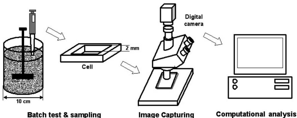
Figure 1 | Schematic illustration of image capturing and analysis procedure.
