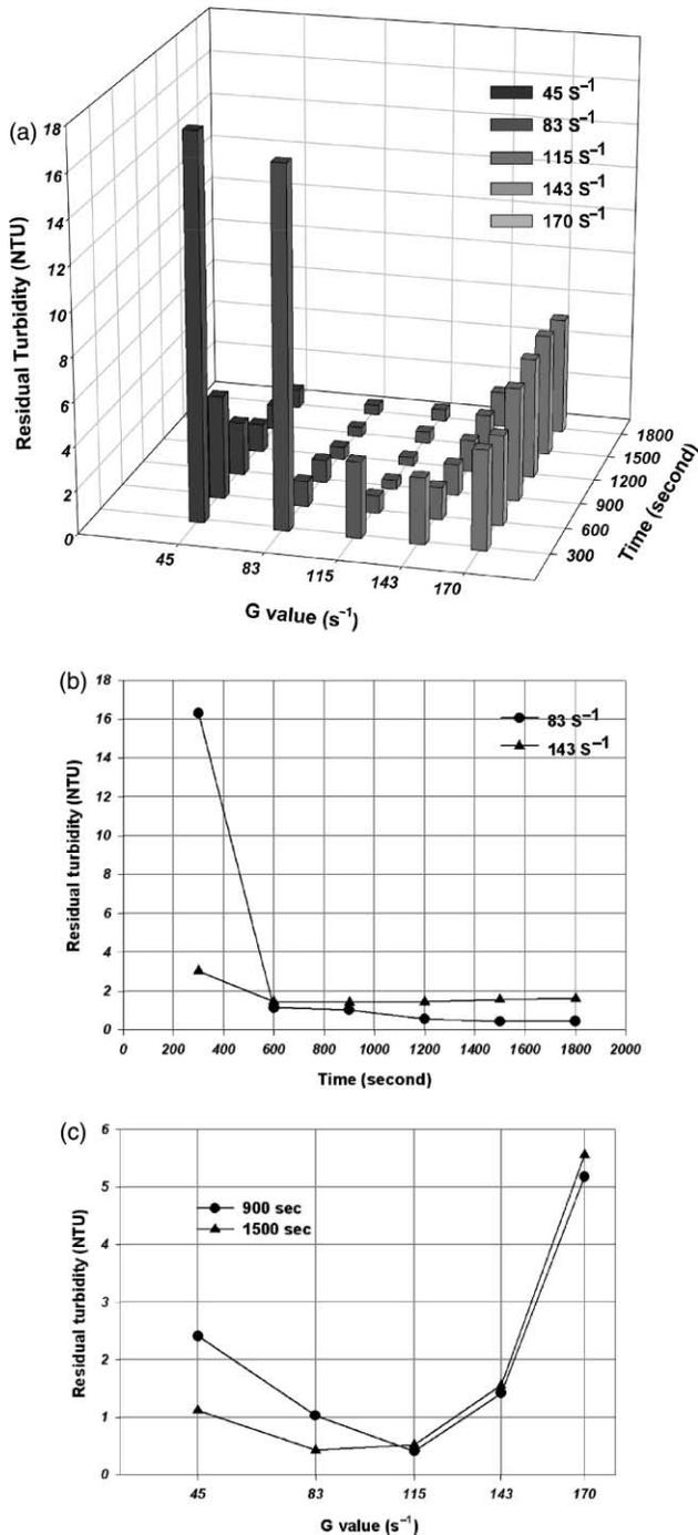
**Figure 3** | Turbidity at different flocculation conditions in a standard jar test. (a) Residual turbidity at different flocculation conditions. (b) Relationship between residual turbidity and  $t$  value (at 83  $s^{-1}$ , 143  $s^{-1}$ ). (c) Relationship between residual turbidity and  $G$  value (at 900 s, 1,500 s).
