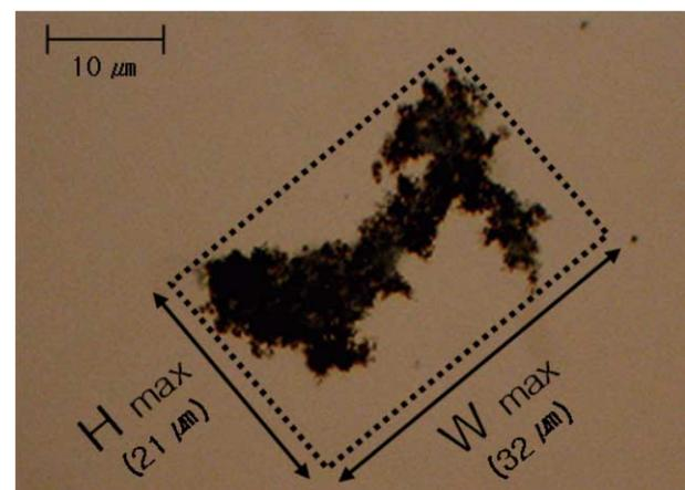
Figure 2 | Definitions of longest width and height for Feret Diameter.
