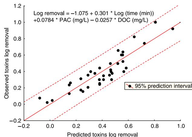
**Figure 2** | Predicted cyanotoxins (anatoxin-a and microcystin-LR) removal by powder activated carbon (PAC) application according to contact time, PAC dosage and dissolved oxygen concentration. Adapted from Mouchet & Bonnellye (1998), Cook & Newcombe (2002a,b) and European Commission under the Fifth Framework Programme and contributing to the implementation of the Key Action “Sustainable Management and Quality of Water” (2005).
