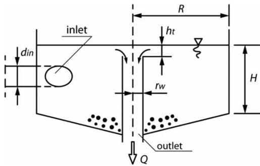
Figure 1 | Schematics of axial cross-section of HDVS.
