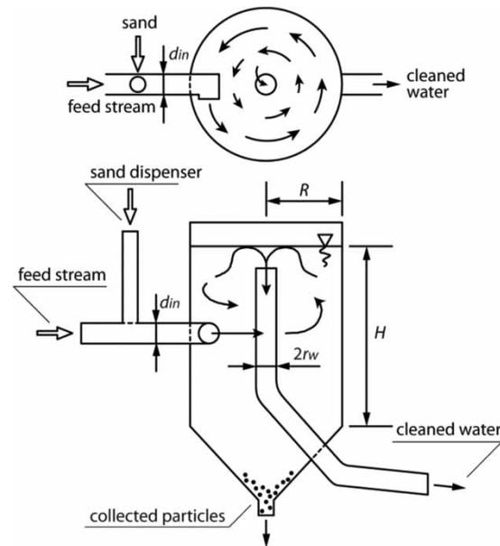
Figure 2 | Schematic of the laboratory separator.
