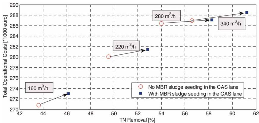
**Figure 4** | Costs and TN removal while varying the influent flow to the MBR system. Scenarios with MSS and without MSS operations have been compared.
