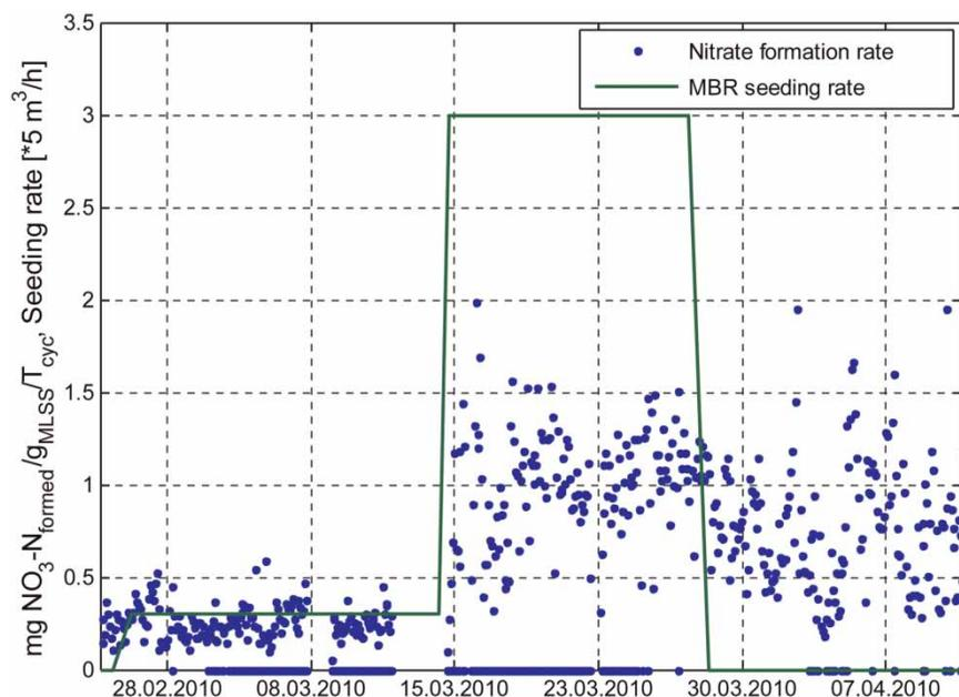
Figure 3 | Measured specific nitrate formation rate in the CAS aeration tank during MSS operations. The MBR seeding rate is also reported.
