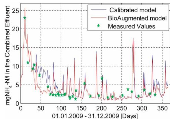
**Figure 2** | Modelled versus measured soluble ammonia in the combined effluent. The effluent ammonia was measured in a year (2009) when no MSS operations were applied. Read '0' as 01.01.2009 and '365' as 31.12.2009.
