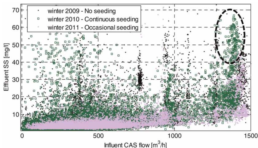
Figure 6 | Effluent SS on-line versus CAS influent flow (2009–2010–2011).
